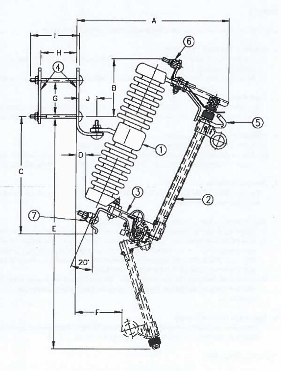
Fig. 1. Arrangement of 33 kV Fuse Cutout.
